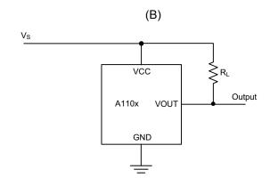
Figure 1: Switching Behavior of Unipolar Switches
