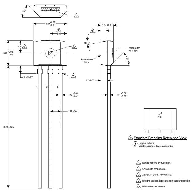
Figure 5: Package UA, 3-Pin SIP (A1106)
