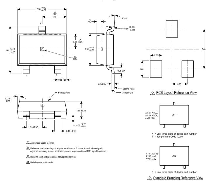
Figure 3: Package LH, 3-Pin (SOT-23W)
