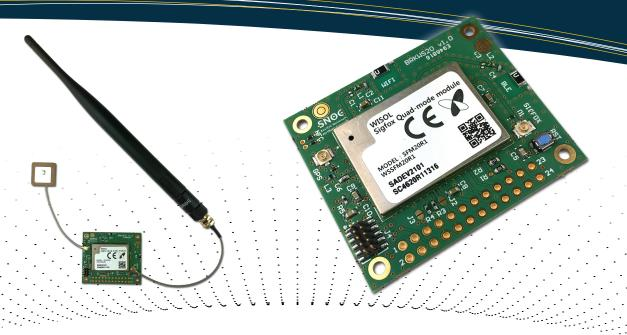
The BRKWS20 breakout board provides an easy way to test under real operating conditions the Wisol WSSFM20R1 quad module. The small size of the board allows you to include it into your real size prototype.
