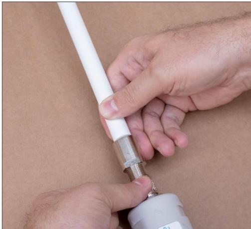
Engage the antenna connector into the LORIX One RF connector as showed on the picture.
