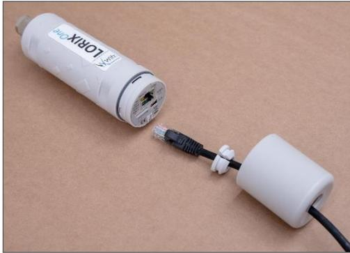
Once the Ethernet cable passed through the cap hole, open the silicon grommet and put it around the cable as showed on the picture.
