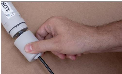
Move the cap in direction of the body while maintaining the cable with the other hand to keep the cable as straight as possible.
