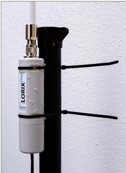
Once the cable and the antenna correctly connected and the LORIX One correctly closed, you can install it on a pole using the 2 provided cable tie.
