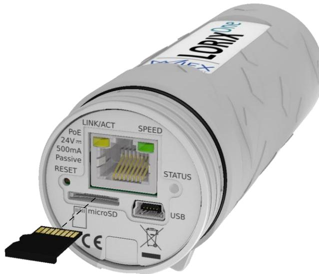
To insert an SD card, simply push it into the hole until it makes a “click” sound. To remove the card, simply push it back until you hear the “click” sound. The SD card will come out on release.
